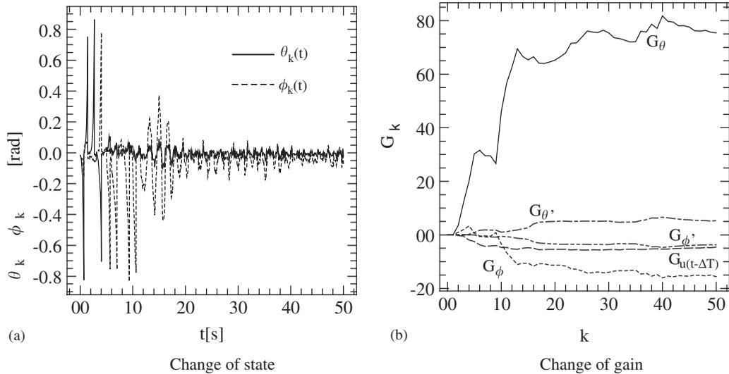
Figure 2. Learning control of a physical pendulum system. (a) Change of the state, (b) change of the gain.
